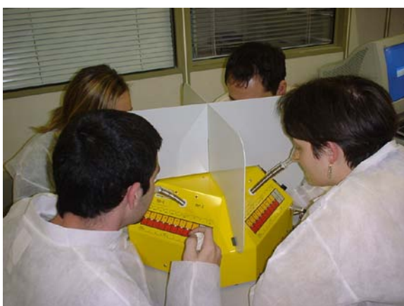
Figure 4 : Olfactometric working sessions according to the AFNOR NF EN 13725 standard
