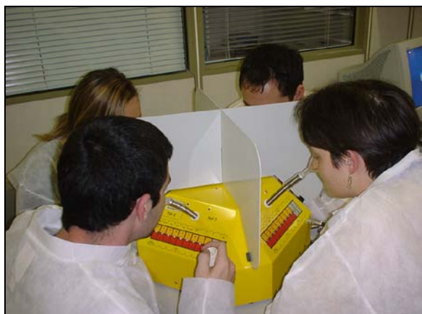
Photo 2: Olfactometric tests according to the AFNOR NF EN 13725 standard
